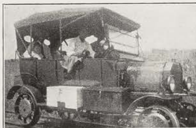
RAILROAD TRIP IN PHILIPPINES This Ford car with iron wheels and lunch box on the side, is locomotive, coach, and dining car all in one
